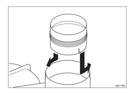
The reducing collar must be used in recirculation mode. Place the collars into the exhaust connections and turn left to lock them in place. Do <u>not</u> insert the non-return flaps.
